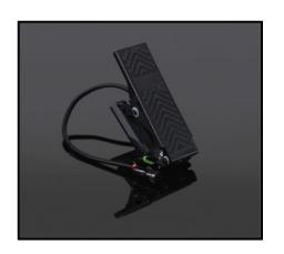
Orscheln Products Electronic Throttle Pedals deliver a precise signal that interacts with the engine's electronic fuel management systems. The fast-reacting pedal provides smooth driver operation and features a durable, longer-life programmable Hall Effect sensor. Polymer components create a lightweight pedal, as much as half the weight of current pedals in the marketplace. Quality testing ensures reliability and durability.
